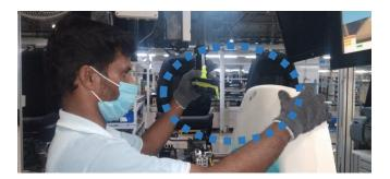
Seat Assembly Line operator scanning barcode to confirm correct part Number usage
