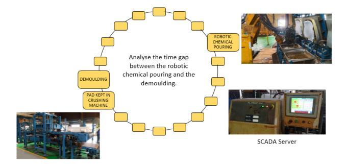
The above carousel image depicts a continuous line with 18 Carriers at Spack Chennai Plant. The line runs at a pre-fixed speed (Cycle time), set to get the best results in terms of pad production, which is based on the chemical reaction and cure time.
