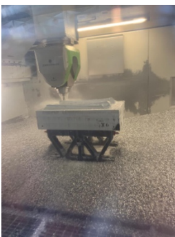
Machining of an Arm Rest mould on a 5 Axis VMC
